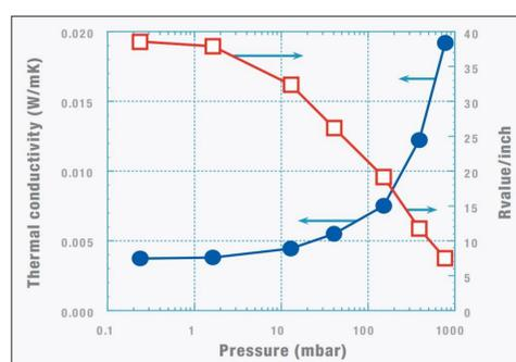
Graph 1: Pressure vs Thermal Conductivity
