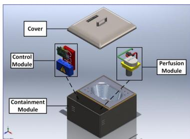
Figure 1: Expanded SolidWorks Model
