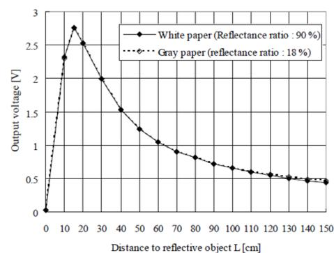
Figure 8: Output Voltage vs Range of distance
