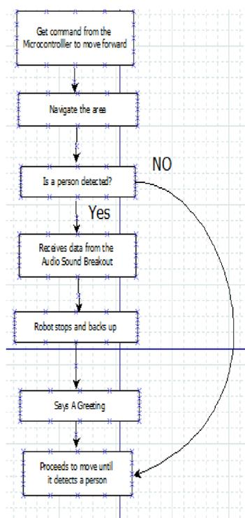
Figure 3: Control Flow Diagram
