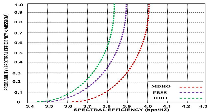
Fig.4. Cumulative Distribution Function (CDF) of Average Down-Link (DL)
