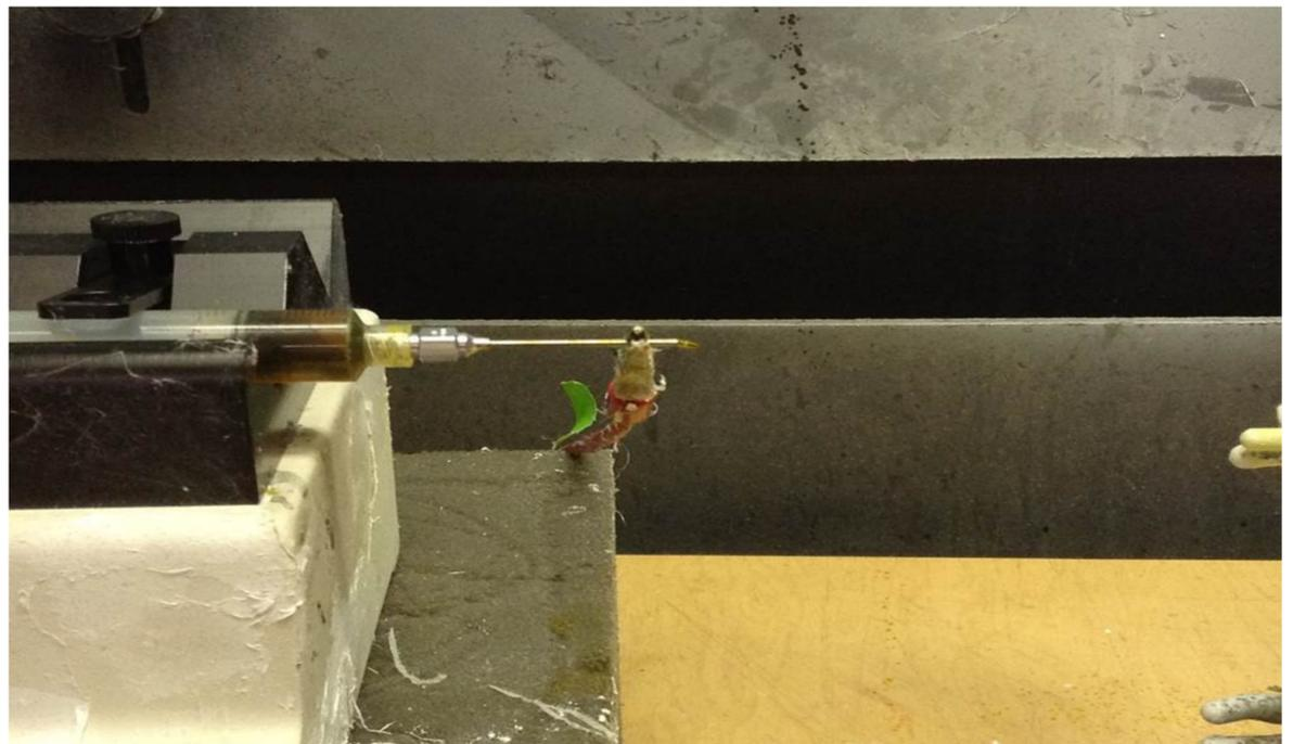
Fig 2. electrospinning process of flavin mononucleotide (FMN) and single-walled carbon nanotubes (SWNTs)
