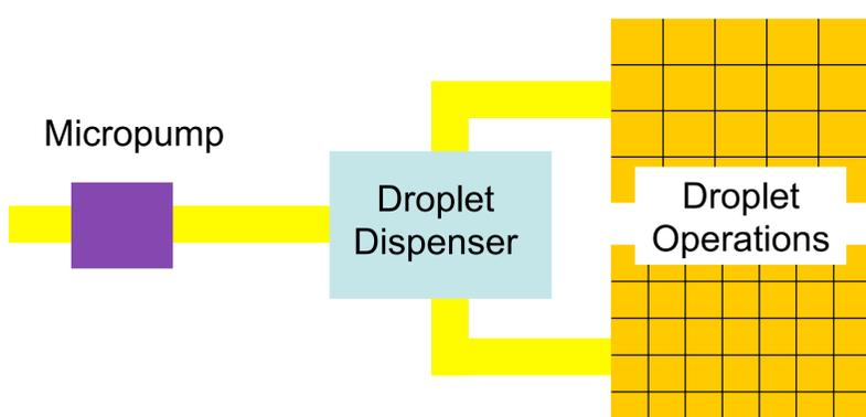
Fig. 2. High-throughput Microfluidic Droplet Dispenser connecting analog microfluidic flow to digital microfluidic biochip (DMFB)
