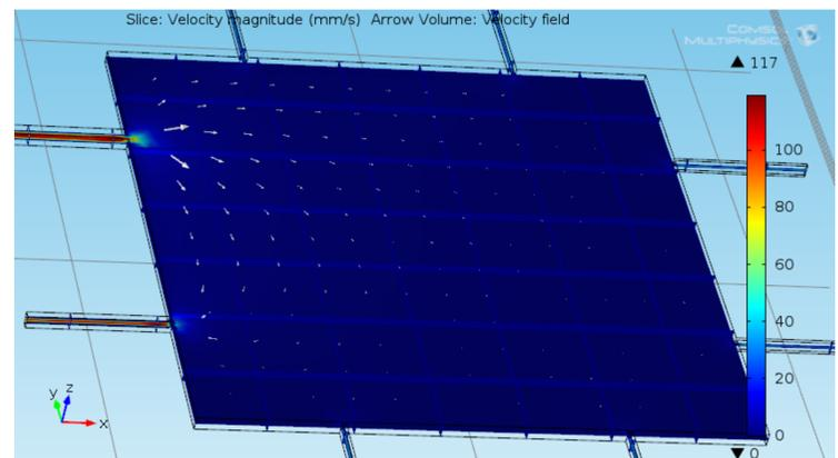
Fig. 3. COMSOL simulation of velocity field of microfluid inside dispenser
