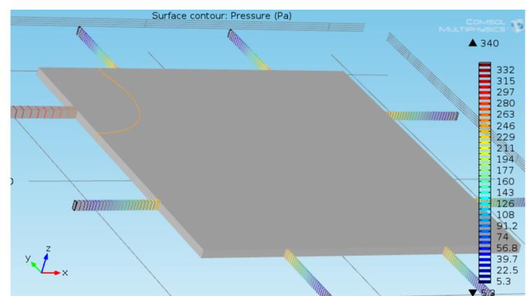
Fig. 3. COMSOL simulation of pressure distribution inside the dispenser
