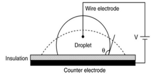
Fig. 3. Electrowetting of droplet
