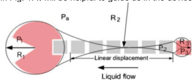
Fig. 4. Theoretical model for droplet dispensing [1]
