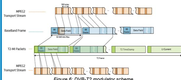
Figure 6: DVB-T2 modulator scheme
