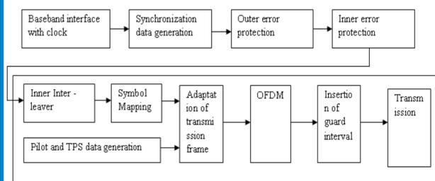
Figure 1: Basic architecture of DVB-T
