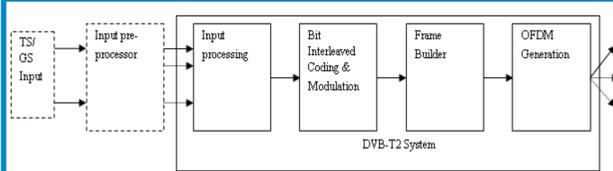
Figure 2: Basic architecture of DVB-T2
