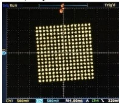
Figure 3: Rotated constellation for 256 QAM at receiver
