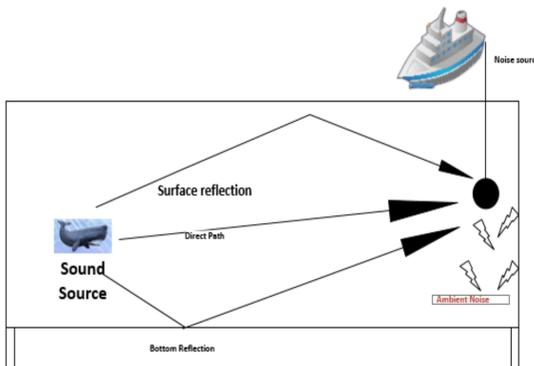
Figure 1.2: Diagram showing underwater multi-path propagation
