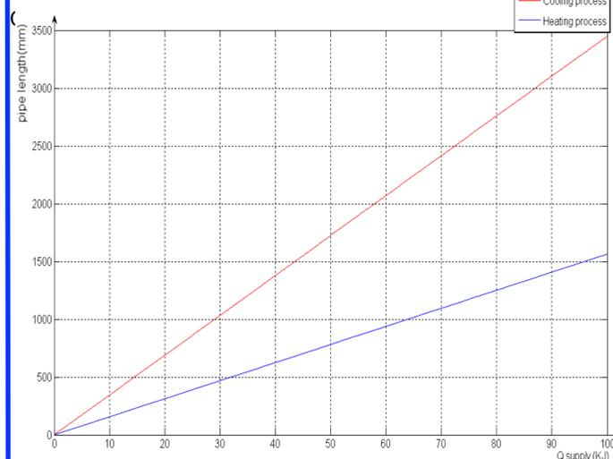
figure2: length requirements of the heat and cool process
