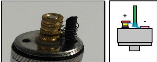
**Figure 1:** The image on the right is a diagram of the components of an electronic atomizer. The green section is the wick fabricated from a rolled stainless steel mesh. The light blue helix is the heating element, which heats the coil once a current is introduced through the lead screws. The grey section is the reservoir that contains the liquid that will be vaporized. The image on the left is the actual product represented by that diagram.
