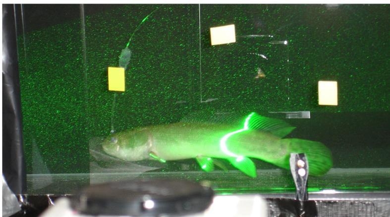
Figure 2: Photo of PIV being used during the feeding of the Amia fish
