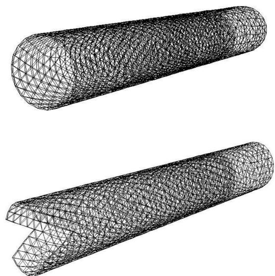
Figure 7 & 8: Image of generated mesh for planar and wedge shaped mouth in Fluent
