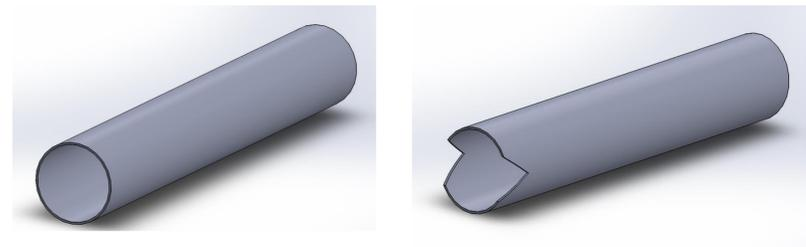
Figure 5 & 6: Image of Planar and Wedged shaped mouth geometries.
