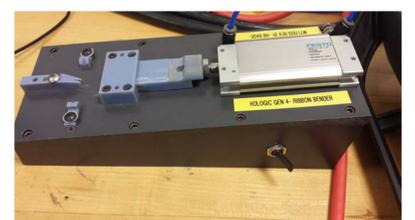
Figure 13: Ribbon bending device
