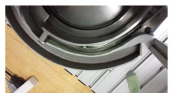
Figure 9: Ramp to guide ribbons to exit chute
