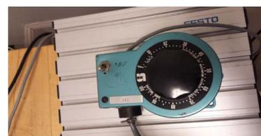
Figure 10: Voltage Controller for Rotational Feeder
