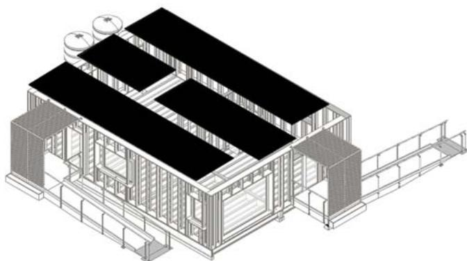
Figure 3: DT90 Roof Mounted Solar Panels (shown in black)
