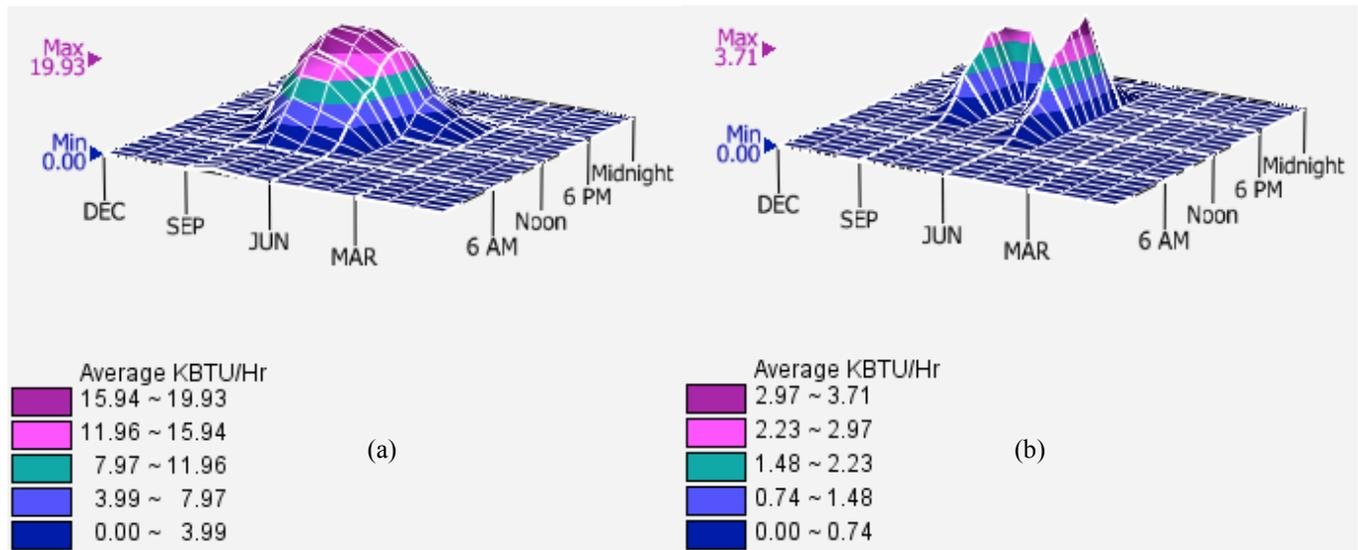
Fig. 3. HEED results displayed in a 3-D graph displaying months of a year, hours of a day, and the power demand of the air conditioner system between a comparison among two Cases (Case 1 and Case 9). Note the changes in maximum output and curvature due to introduction of window eaves, automated shades acting during the warmest summer months, combined with an increase in insulation.
