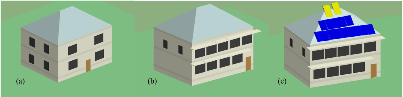
Fig. 1. A visual representation of energy efficiency design measures employed and tested by different scenarios. (a) Baseline window and door layout, east facing side (b) Case 2 with window and door layout reconfigured to face south, with protruding eaves on top of windows (c) South facing side of Case 8 showing PV and solar hot water panels applied to the south facing side only of building roof
