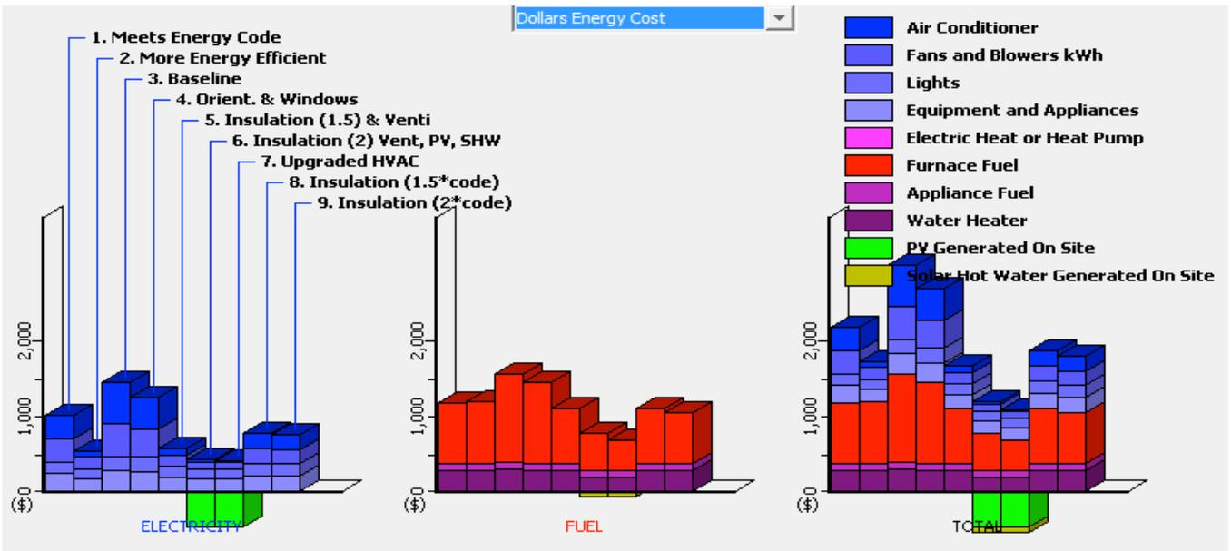
Fig. 2. Graphical display for energy cost of nine cases considered in the study, with electricity and fuel cost shown separately as well as together for total cost
