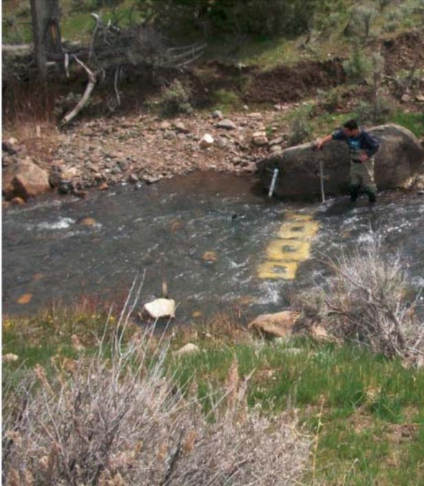
Figure 1. Birkbeck Bedload Sediment Trap Boxes at the Reynolds Creek Experimental Watershed.
