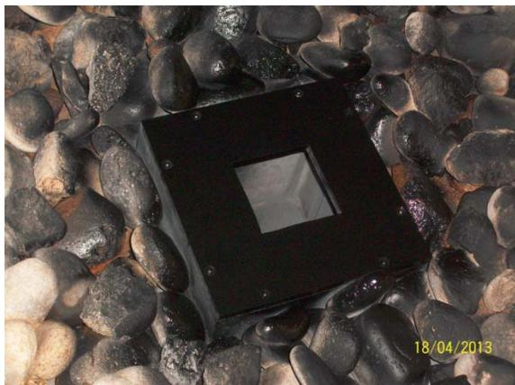
Figure 3. Sediment trap Model 1 shown empty (Birkbeck type)
