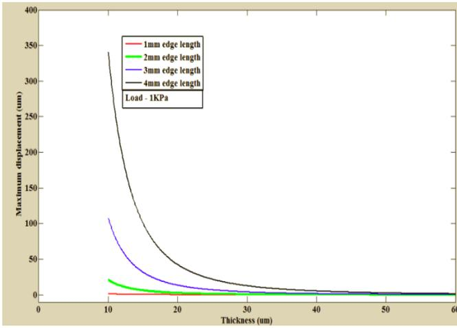
Fig 5. Maximum displacement vs. thickness characteristics of diaphragm
