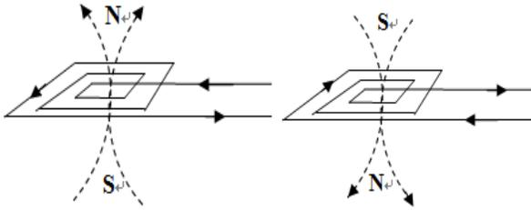
Fig 3. Control of north/south poles of electrical coil by switching the direction of current.
