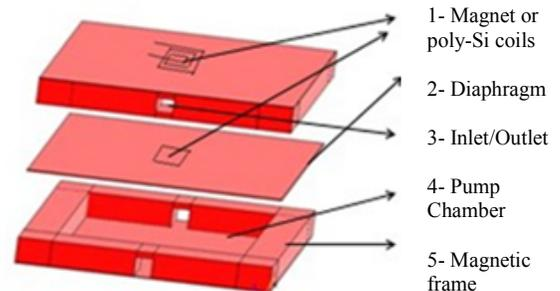
Fig1. Structure diagram of the magnetic tri-membrane micropump
