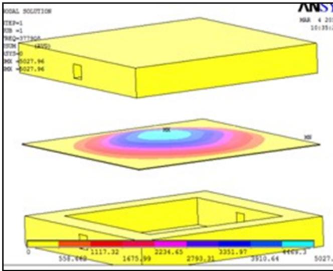
Fig 12. Stress contour plot of the central membrane
