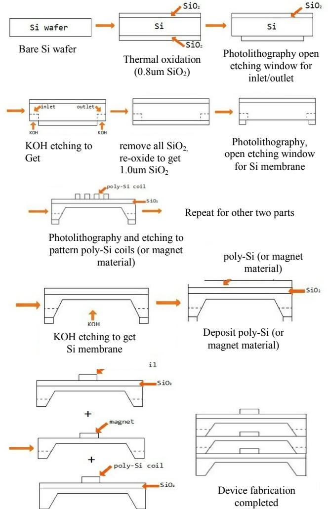
Fig 13. Fabrication flow of the micropump (cross-sectional view)
