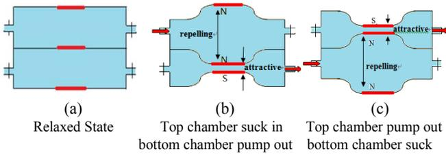
Fig 2. Working principle of the tri-membrane micropump
