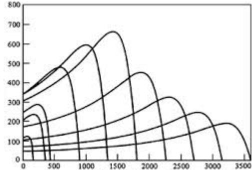
Fig. 10. Induction machine torque vs. frequency characteristics
