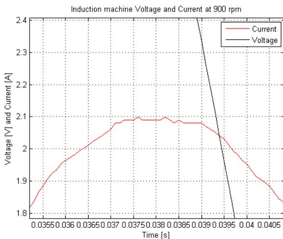
Fig. 12. Presence of 19<sup>th</sup> current harmonic in the Induction machine current vs. time snapshot at  $f = 30$  Hz
