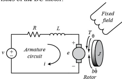
Fig. 1. Permanent magnet DC motor equivalent circuit
