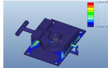
Fig 4.3 FEA of fixture while cutting
