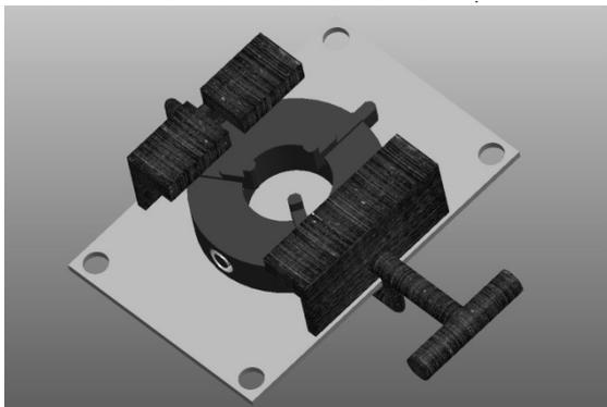
Fig IV.1 Fixture for shaping, milling and drilling
