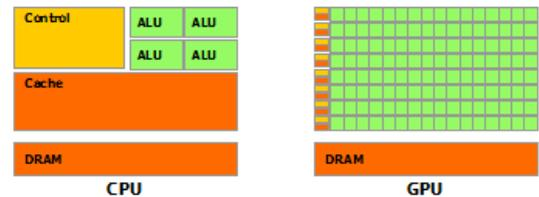
Fig. 1: CPU vs. a GPU ([www.nvidia.com](http://www.nvidia.com)).
