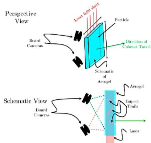
Figure 2 Baseline payload schematic.
