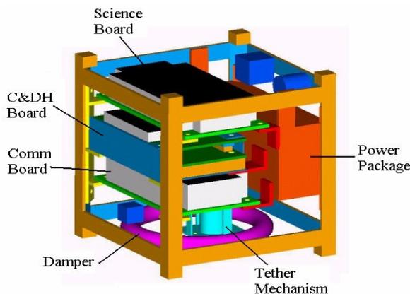
Figure 1. Internal Configuration
