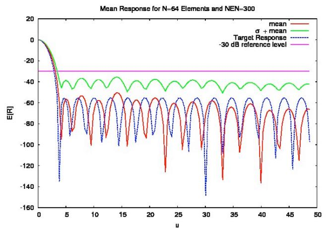
Fig. 6. Expected Beam Pattern and one  $\sigma$  deviation for Nonuniformly Distributed  $x$
