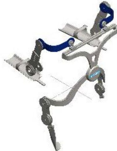
Figure 1: Full CAD drawing of the Exoskeleton Suit
